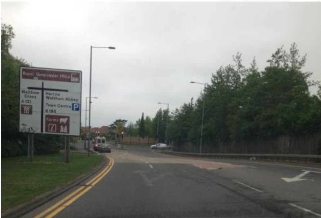
Figure 5: Meridian Way approach showing bifurcation arrow at start of lanes. Arrow to be reversed to indicate 'ahead' direction is via right hand lane
